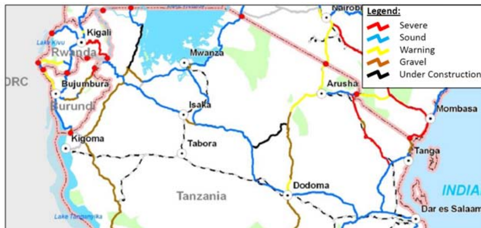
Figure 3-6 Condition of Central Corridors Roads
