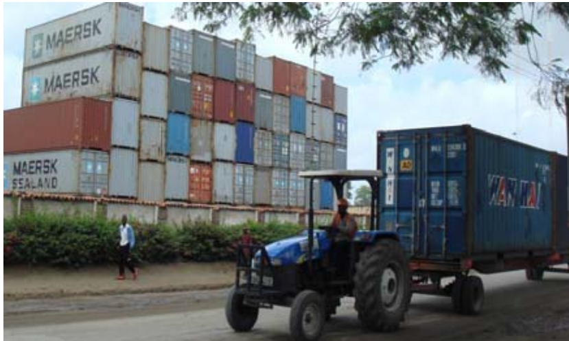
Figure 5-1 Use of Tractor for Container Transfers
