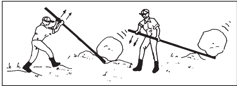
FIGURE 3-E2.4 BOULDER REMOVAL BY LABOUR USING CROWBARS
