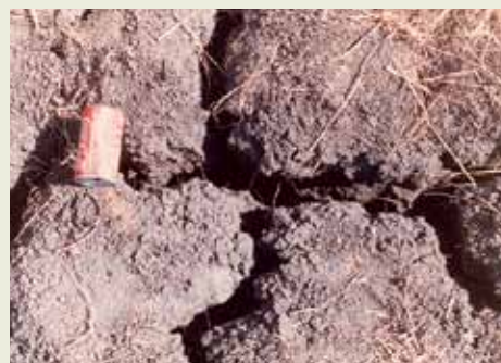
Expansive “black cotton” soil exhibiting wide-spaced shrinkage
