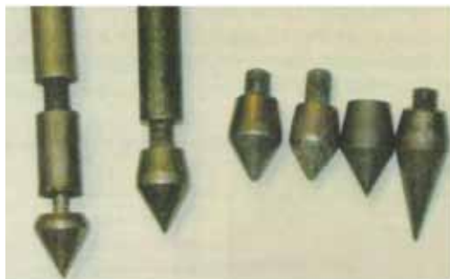
Photo 2A-1: Typical cones and problems
