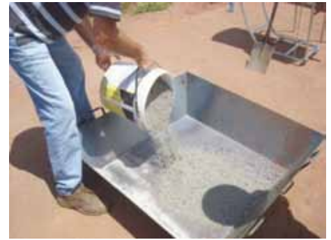
Batching of aggregates
