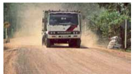
Dust generated by unpaved roads
