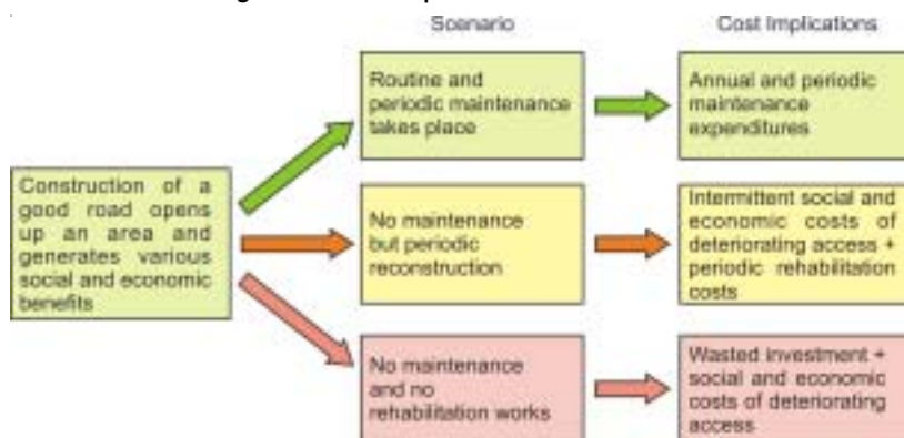
Figure 3.5 Cost Implications of Maintenance
