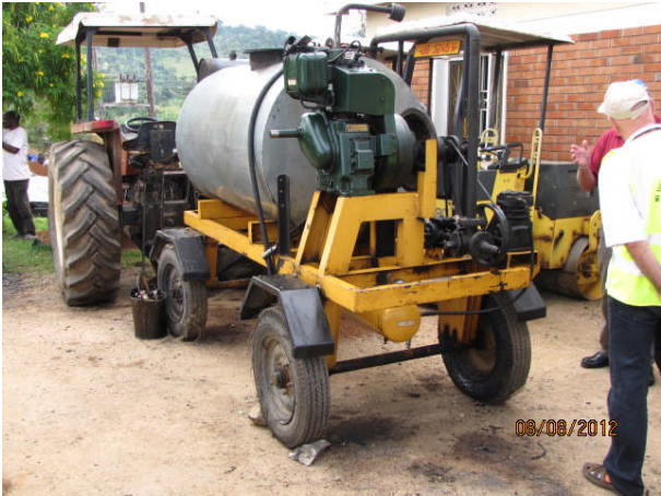
(a) Motor powered pump and hand lance sprayer (b) Bitumen distributor with heating device
